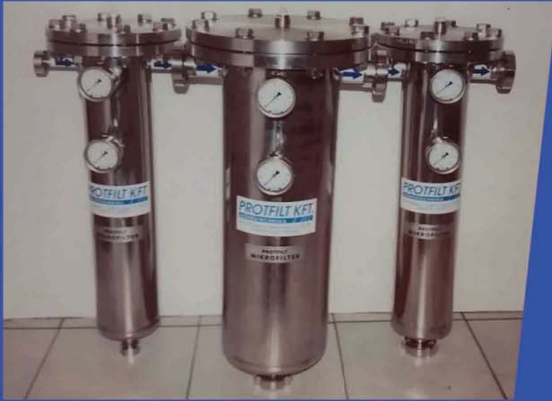
Completely stainless steel filter unit for acidic media (Unilever plant)
