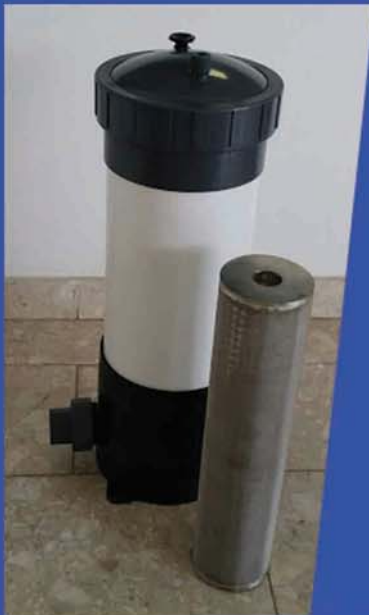
Industrial plastic filter housing with sieve for alkaline media (Hungarian chemical plant)
